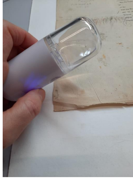
Flattening of areas of creases and local deformations after water misting with the nano-mister.
